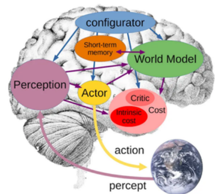
Figure 2 The modular architecture of an objective-driven world model based on LeCun's 2022 framework. It uses an internal simulation layer to predict environment changes and minimize cost before taking action. [1].
