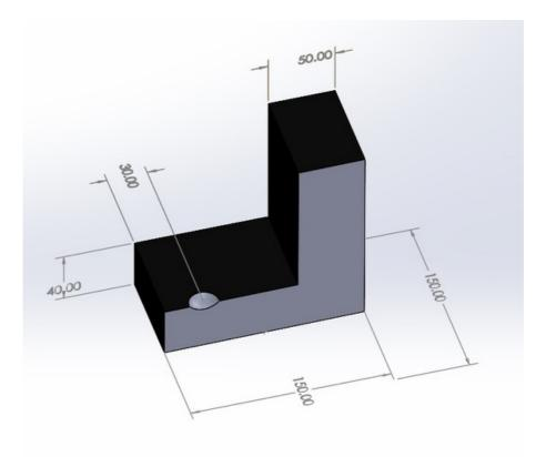
Figure 1.11 - **Cross section** of Stone holder (dimensions in **mm**)
