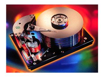
A computer's hard drive is a device consisting of several hard disks, read/write heads, a drive motor to spin the disks, and a small amount of circuitry, all sealed in a metal case to protect the disks from dust. In addition to referring to the disks themselves, the term hard disk is also used to refer to the whole hard drive.
