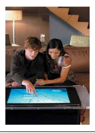
Surface uses a series of infrared cameras (five to be exact) to virtually see objects placed on top of it, hand gestures and touch. This user input is then processed and the result is displayed on the surface using rear projection. It sounds simple but actually its not!
