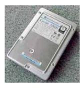
current disks use a cobalt-based alloy. Hard disks are flat, circular plates made of aluminum or glass and coated with a magnetic material. Most hard disks are "fixed disks," which have platters that
